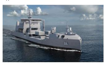
HMNZS Aotearoa will be a world-first naval "Environship", with Hyundai using the Rolls-Royce Environship concept design under licence. The design incorporates a new wave-piercing hull, which reduces resistance and lowers fuel use, while its combined diesel electric and diesel propulsion plant has lower fuel emissions than older vessels.
